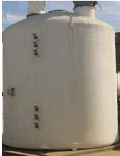
Figure 8 – Sample Carbon Vessel for Hg Removal 6
